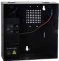
ME-0515M Multipurpose Power Management Enclosure • Two isolated output channels: 12 VDC at 2 Amp (4 Amps total) • Power Management Board with 7AH Lead Acid battery charger • Universal Input Voltage 100 VAC to 240 VAC 50/60Hz auto select • Tough metal enclosure featuring QXR's PowerLock™ C13 socket
